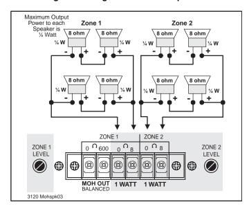
Fig 27B - Using four 8 ohm Speakers
